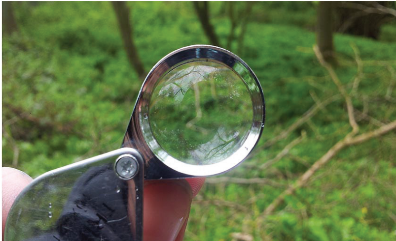
Figure 1. Geological hand lens
