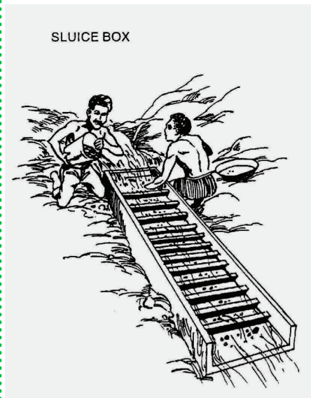
Figure 1. The sluicing method of mining. Image courtesy of PNG Chamber of Mines and Petroleum.
