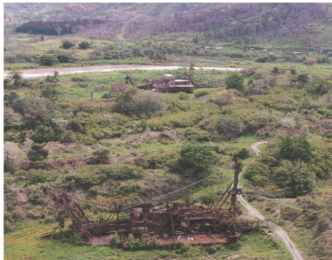
Figure 2. Remnants of dredging equipment used for mining in the Morobe goldfields in the 1960s. Photo courtesy of PNG Chamber of Mines and Petroleum.
