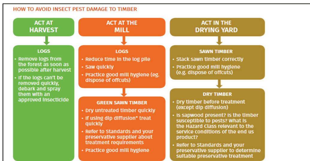
Figure 1: How to avoid insect pest damage to timber *BFCA is sometimes used in PNG to treat freshly-sawn green timber by dip diffusion.
