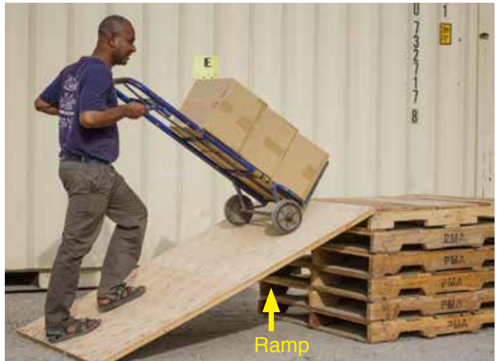
A ramp helps move boxes easier.
