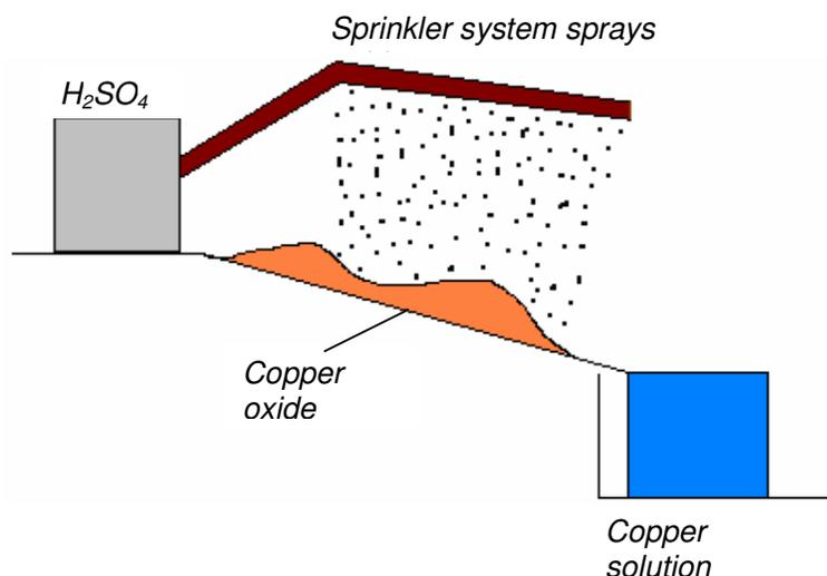
The copper oxide ore is dug out of the ground and sprayed with acid. The acid leaches (soaks) through the ore and reacts with copper oxide. The resultant copper solution is collected in a tank at the bottom of the ore heap.
