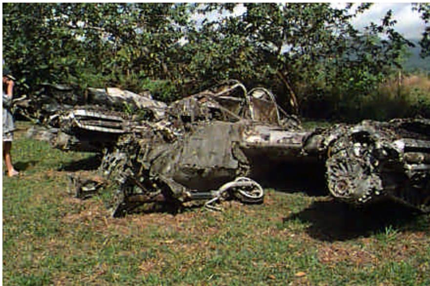
Figure 4. A World War II plane wreckage. The aluminium has withstood the effects of weathering as it does not react very well with air.
