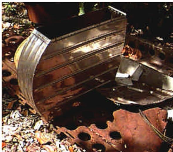
Figure 6. This World War 2 ammunition magazine made from high grade stainless steel. It has not rusted after almost 60 years.
