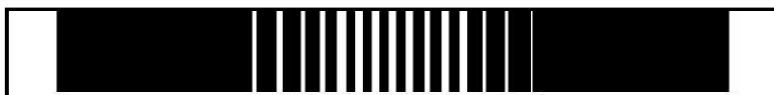
Figure 26: The interference pattern produced by light incident on a pair of closely spaced slits.
